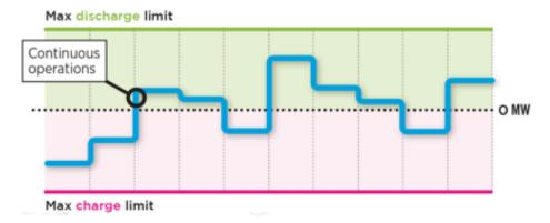
Charge mode - shall mean the mode of operation of an Energy Storage Resource model
