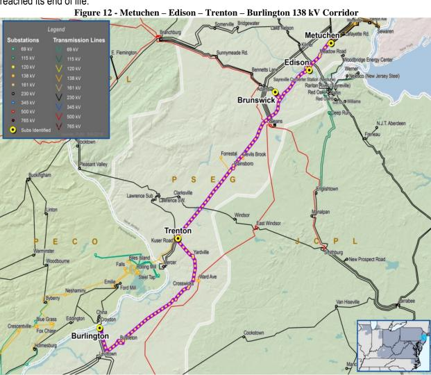
Three alternatives were considered to address the issues identified on the Metuchen – Burlington 138 kV corridor. The first was to remove the corridor without replacement. The second was to install new parallel circuits on a new right of way and remove the existing corridor. The third was to replace / rebuild the corridor in with new foundations, and hardware designed to either 138 kV or 230 kV.
