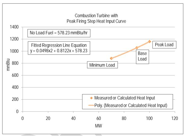
Each diamond in the graph above is a design heat input data point obtained from the original equipment manufacturer or calculated by heat balance. A regression analysis was performed on the design data to obtain the unit's Heat Input curve as a function of Output with natural gas as a fuel:
