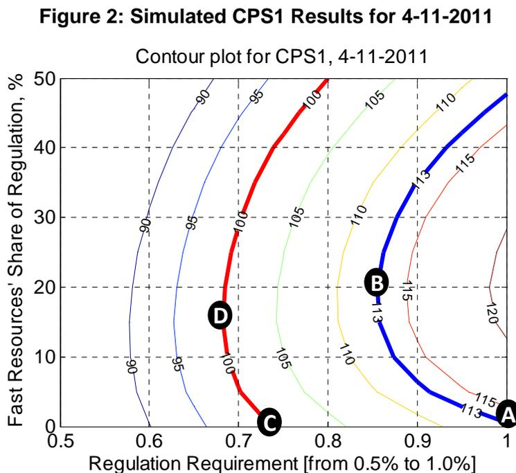
The contours provide insights into the trade-off between reducing the Regulation Requirement and increased use of Fast Resources. The curves in Figure 2 suggest that it is possible to reduce the Regulation Requirement while still being CPS1-compliant to a point.
