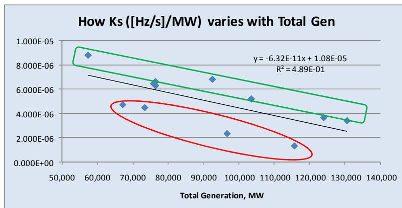
**Figure 8: Estimated System Inertia based on empirical data.**
