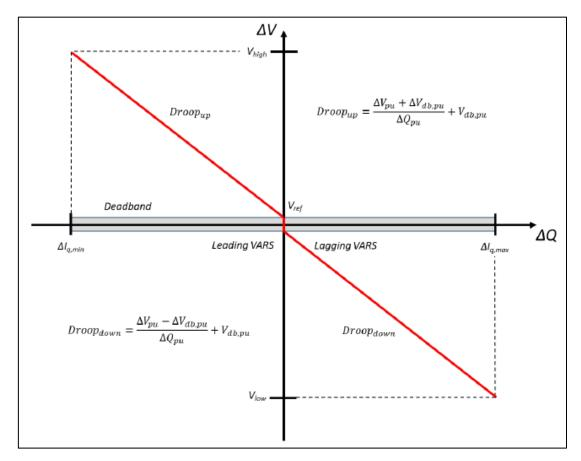
Figure 4. Reactive Power – Voltage Control Characteristic
