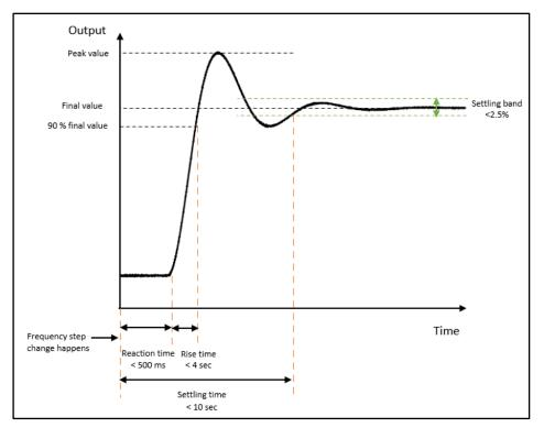
Figure 1. Dynamic Active Power-Frequency Performance
