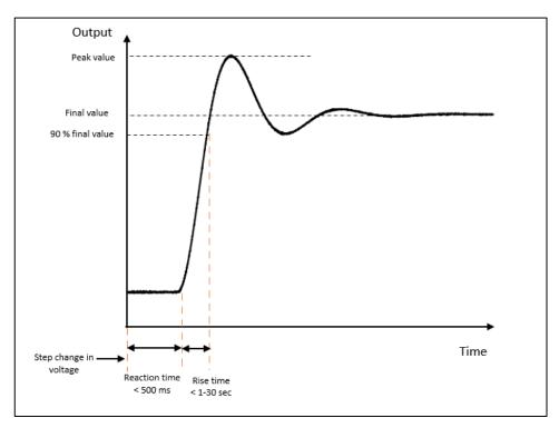
Figure 2. Small Disturbance Reactive Power-Voltage Performance
