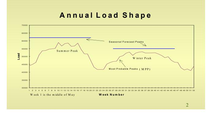
Diagram 7 – Load Shape combined with Weekly Load Distribution
