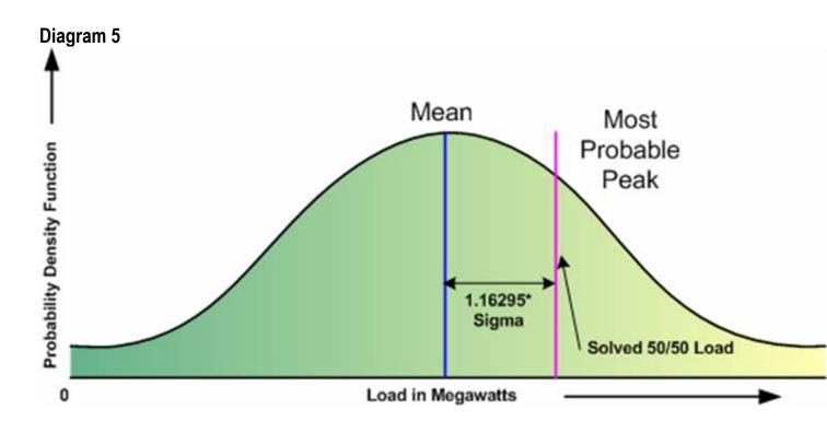
Diagram 7 emphasizes the point that each weekly load point on the annual load shape does not represent a single value, but is itself the most probable peak drawn from an entire distribution of possible peaks. A load distribution similar to the one depicted in Diagram 5 is associated with each weekly peak plotted in Diagram 6. This approach ensures that every possible load level, not just the expected or average load level, is considered in our adequacy analysis.
