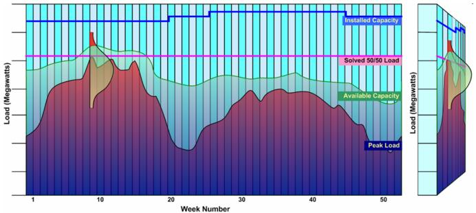
The Green line represents the Available capacity. The tail of the weekly load distribution shown above the green line represents a loss-of-load event. Picture this diagram in 3 dimensions with the bell shape load extending up out of the page as shown in the image to the right.
