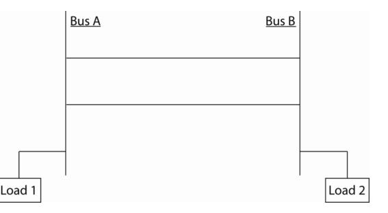
$$P_{R} = (V_{S}) (V_{R}) / Z * \sin^{\delta}$$
