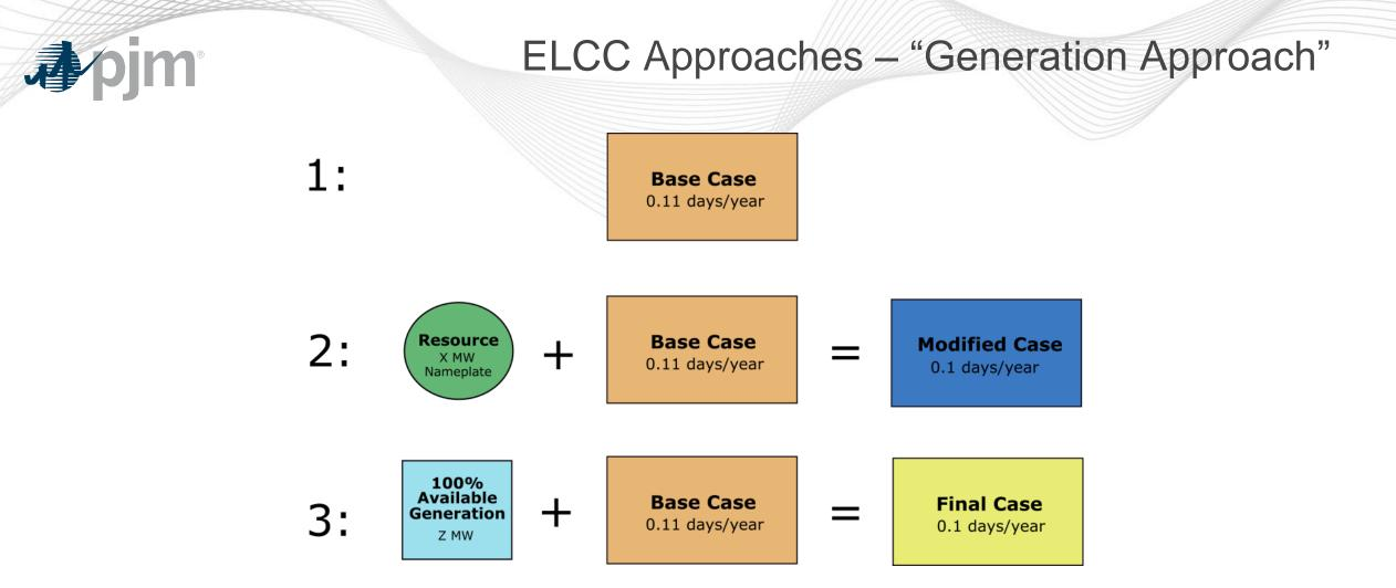
The ELCC of the Resource added in Step 2 is the amount of 100% Available Generation added in Step 3 (Z MW). It can be expressed as percent of the Resource's nameplate (i.e., Z / X)
