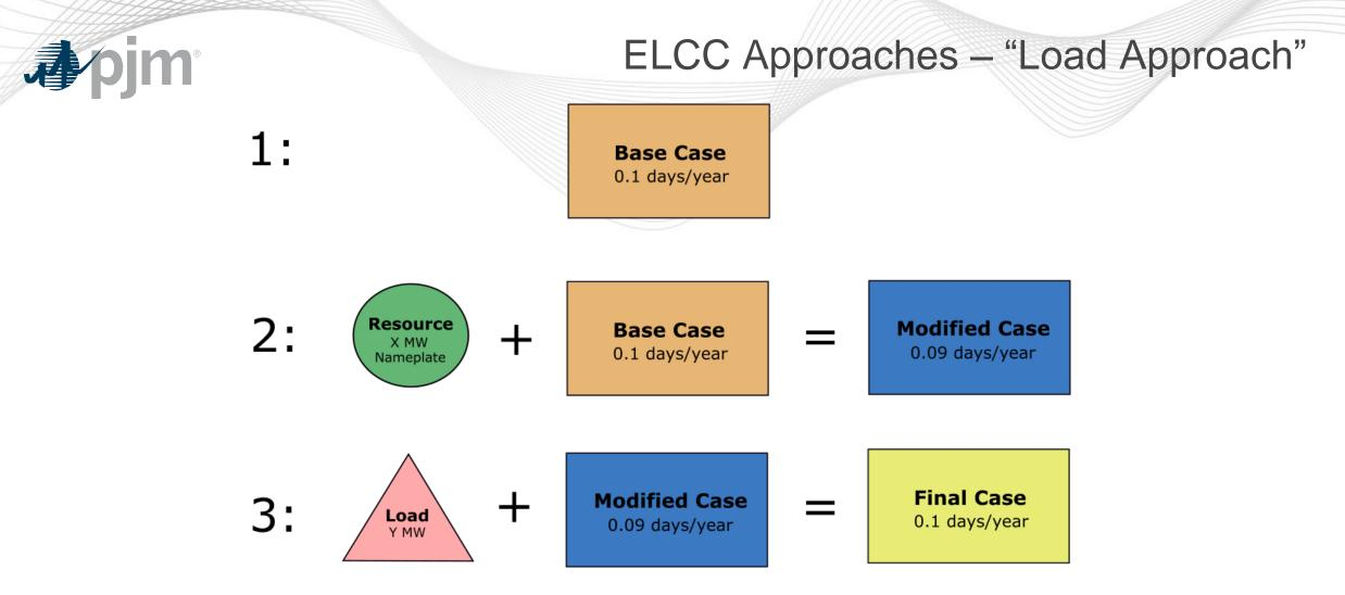
The ELCC of the Resource added in Step 2 is the amount of Load added in Step 3 (Y MW). It can be expressed as percent of the Resource's nameplate (i.e., Y / X)
