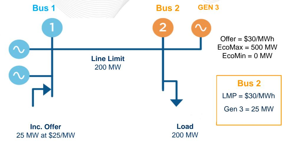
Generator Output Constraint: Gen 1 + Gen 2 <= 150 MW (the Stability Limit)
