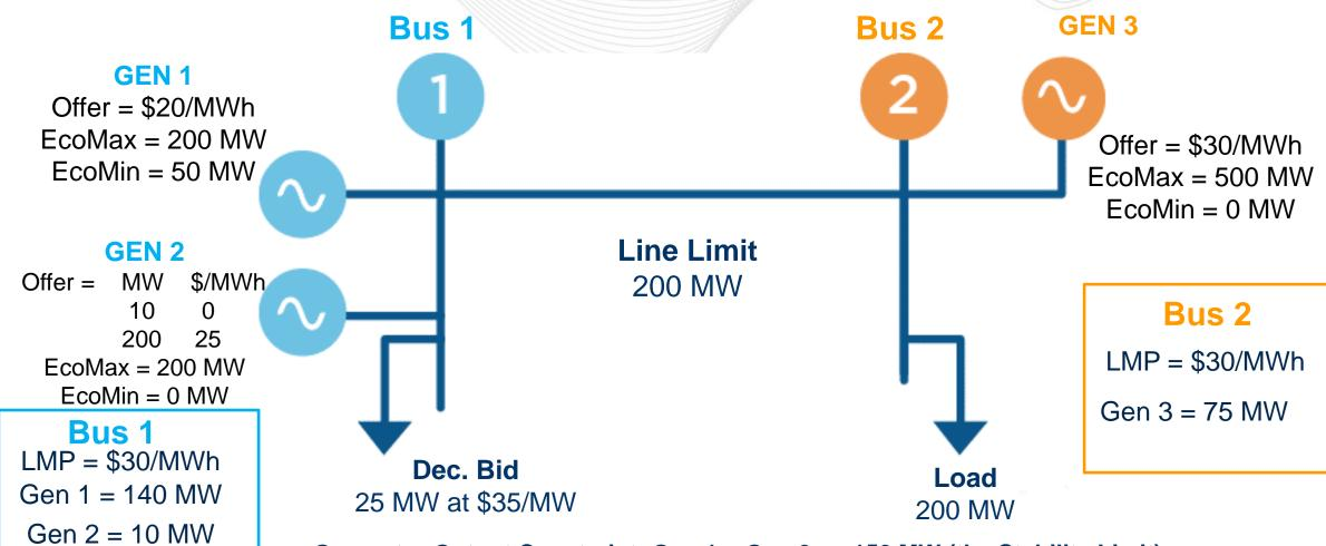
Generator Output Constraint: Gen 1 + Gen 2 <= 150 MW (the Stability Limit)
