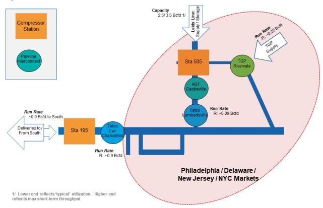
Figure 4-1: Transco Flow Mechanics
