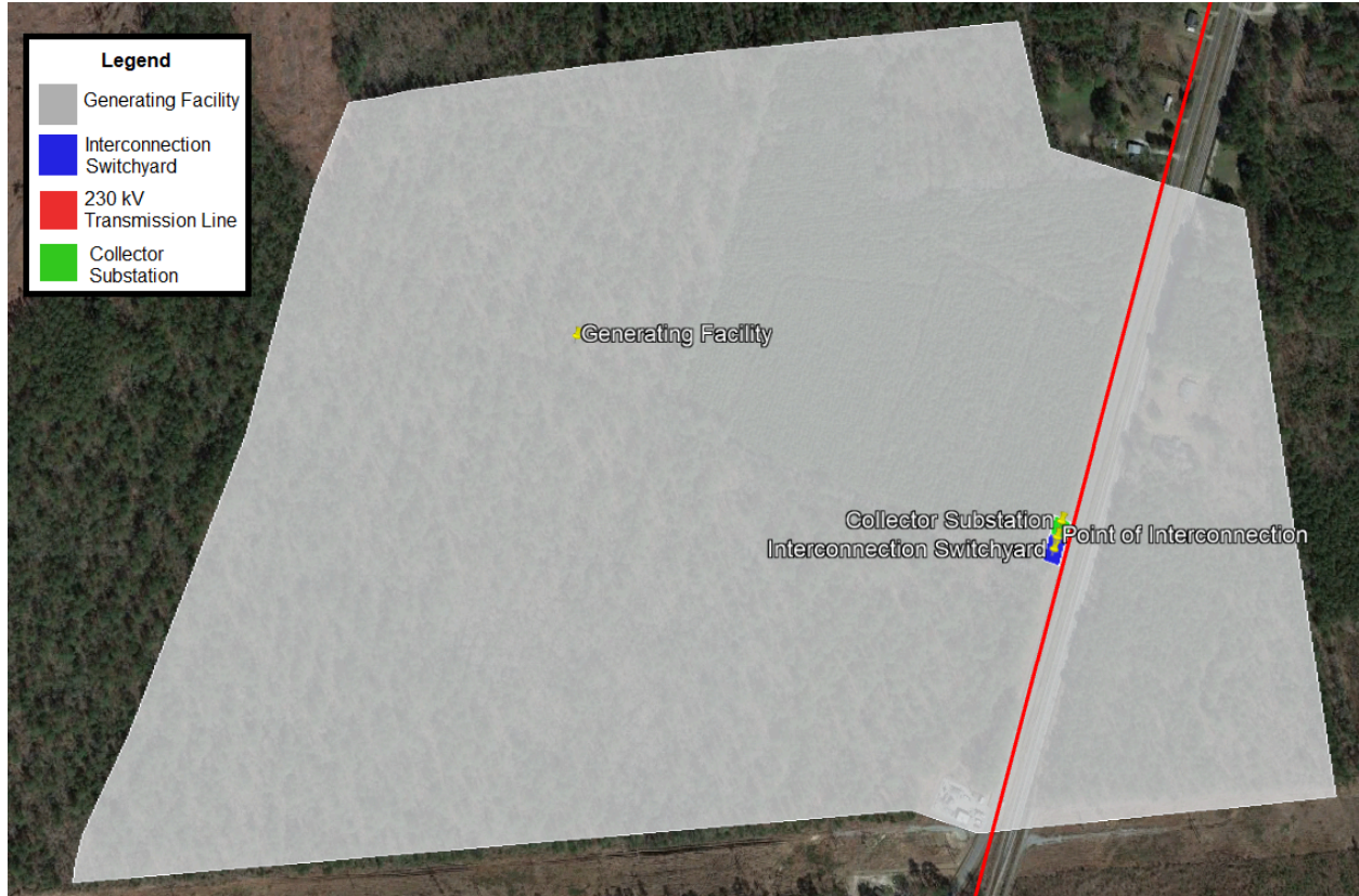
Exhibit 46: Tapping an Existing Transmission Line
