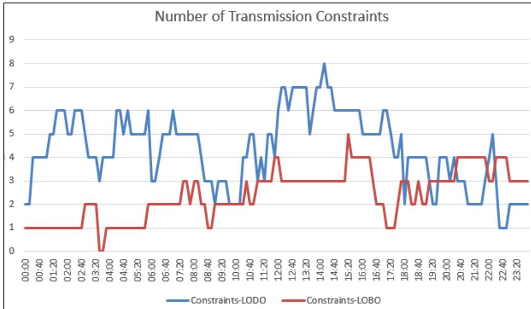
Figure 2-60: Number of Transmission Constraints for Each Interval LOBO vs. LODO, March 28
