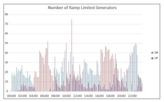
Figure 2-18: Number of Ramp-constrained Units per 10-minute Interval (20% HSBO, March 4)
