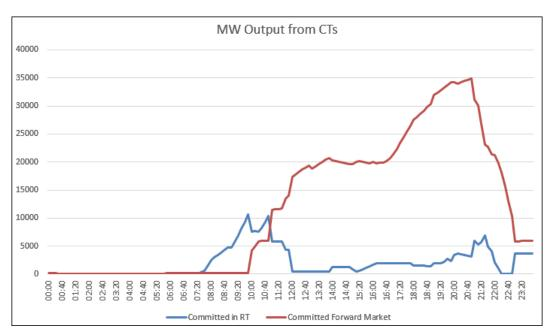
Figure 2-20: CT Dispatch by Interval (20% HSBO, July 28)
