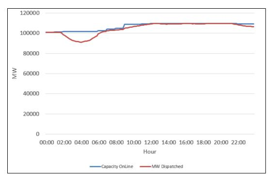
Figure 2-6: On-line Capacity vs. MW Dispatched for Steam + Combined Cycle (2% BAU, July 28)
