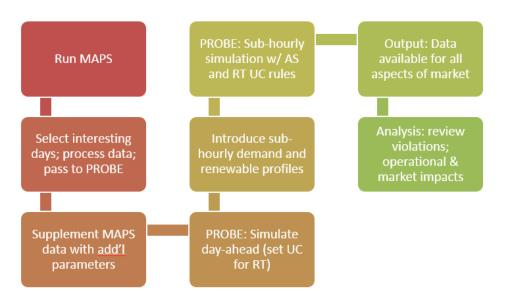
Figure 2-1: GE MAPS-to-PROBE Simulation Process
