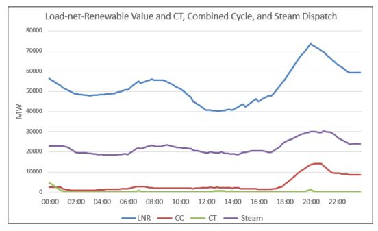
Figure 2-45: Load-net-Renewable with Fuel Generation Dispatch Response (30% HSBO, April 12)
