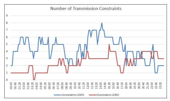
Figure 2-60: Number of Transmission Constraints for Each Interval LOBO vs. LODO, March 28
