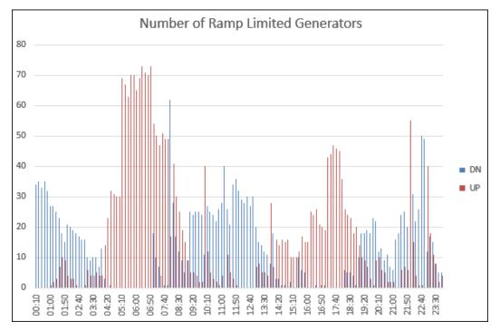
Figure 2-22: Number of Ramp-constrained Units per 10-minute Interval (20% HOBO, January 8)
