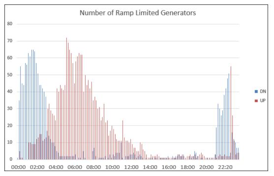
Figure 2-14: Number of Ramp-constrained Units per 10-minute Interval (14% RPS, May 26)
