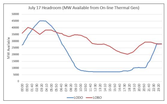
Figure 2-38: Headroom - MW Available from Thermal Generation (20% LODO, July 17)
