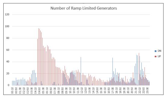
Figure 2-62: Number of Ramp-constrained Units per 10-minute Interval (30% LODO, June 18)
