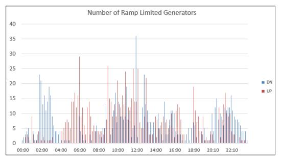
Figure 2-8: Number of Ramp-constrained Units per 10-minute Interval (2% BAU, July 28)
