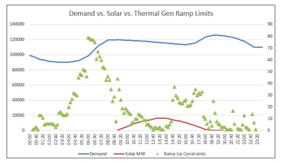
Figure 2-40: Demand MW, Solar Dispatch, and Generator Ramp Limitations (20% HSBO, January 5)
