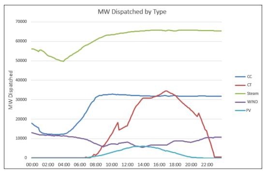
Figure 2-16: Generation by Type for Each Interval (14% RPS, August 3)
