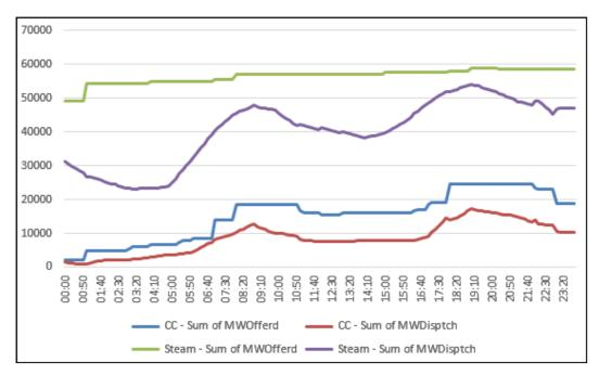
Figure 2-47: Thermal Generation MW Offered vs. Dispatched, On-line Units Only (30% HOBO, January 12)
