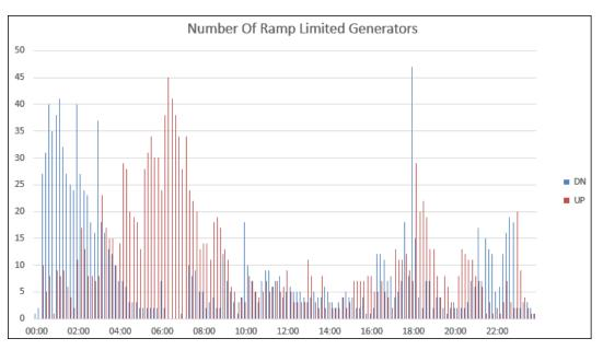
Figure 2-11: Number of Ramp-constrained Units per 10-minute Interval (14% RPS, March 2)
