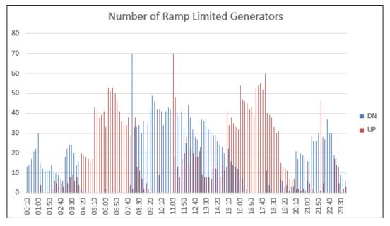
Figure 2-48: Number of Ramp-constrained Units per 10-minute Interval (30% HOBO, March 4)
