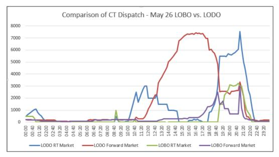
Figure 2-34: Comparison of CT Dispatch for LOBO vs. LODO, May 26
