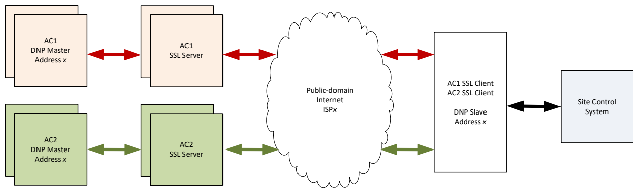
Figure 5. Example Simple Dual-connected Architecture
