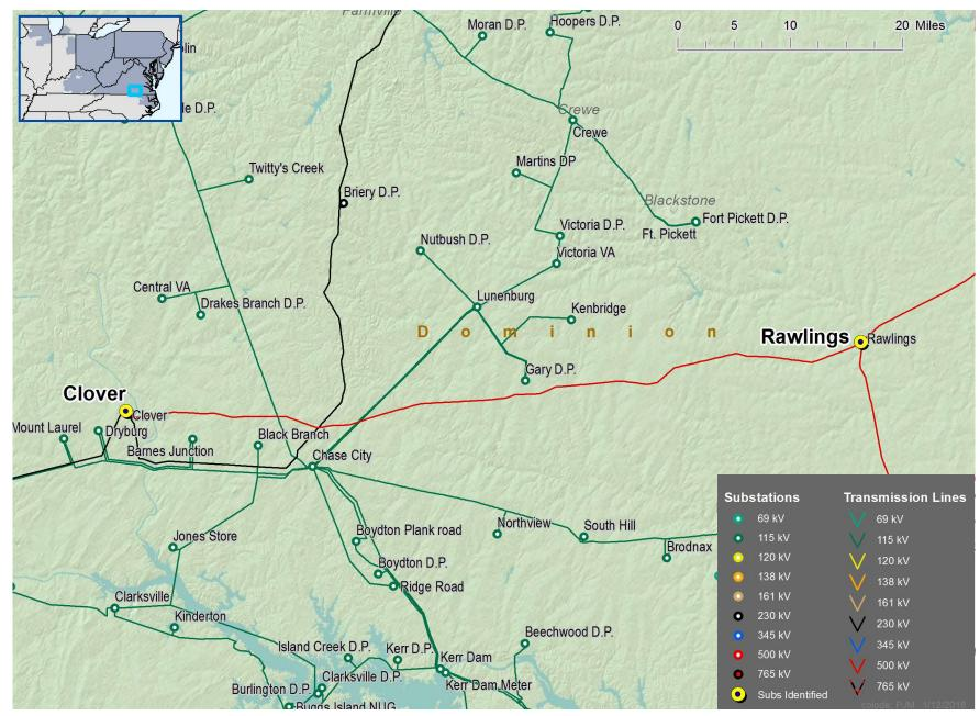
As **Figure 4.2** shows, the solution to install three 500 kV, 125 MVAR static synchronous compensators – two at Rawlings and one at Clover substations (b2978, combined) – adequately reduced voltages to acceptable levels below the 535.5 kV high voltage limit.
