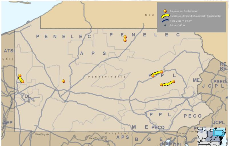
Note: Supplemental projects are transmission expansions or enhancements that are used as inputs to RTEP models, but are not required for reliability, economic efficiency or operational performance criteria, as determined by PJM.
