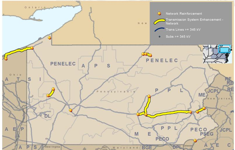
Note: Network upgrades are new or upgraded facilities required primarily to eliminate reliability criteria violations caused by proposed generation, merchant transmission or long term firm transmission service requests.
