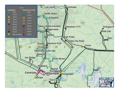
The recommended solution is to rebuild Chesterfield – Centralia 115kV to current standards with a minimum summer emergency rating of 393 MVA. The estimated cost for this project is \$7 million, and the projected in-service date is May, 2020. Dominion will be designated to complete this work.
