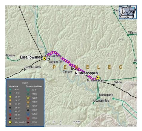
The recommended solution – Baseline Project b3137, rebuilds 20 miles of the East Towanda - North Meshoppen 115 kV line and adjusts relay settings at East Towanda and North Meshoppen 115 kV substations (new rating 202N/245E summer 228N/290E winter). The recommended solution addresses the baseline needs in the area. The estimated cost for this project is \$58.6 million, and the projected in-service date is June 2024. The local transmission owner, Penelec, will be designated to complete this work.
