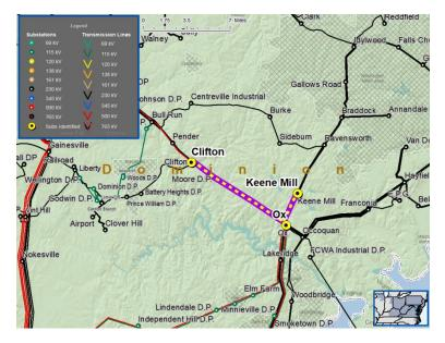
The recommended solution is to rebuild the Clifton – Ox 230kV and part of Clifton – Keene Mill 230kV lines with double circuit steel structures, using double circuit conductor at current 230kV northern Virginia standards, with a minimum rating of 1200 MVA. The estimated cost for this project is \$22 million, and the projected in-service date is December, 2024. Dominion will be designated to complete this work.
