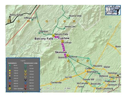
The recommended solution is to rebuild 9.2 miles of Balcony Falls – Skimmer 115kV and 3.8 miles of Balcony Falls – Cushaw 115 kV to current standards with a minimum rating of 261 MVA. The estimated cost for this project is \$20 million, and the projected in-service date is December, 2023. Dominion will be designated to complete this work.
