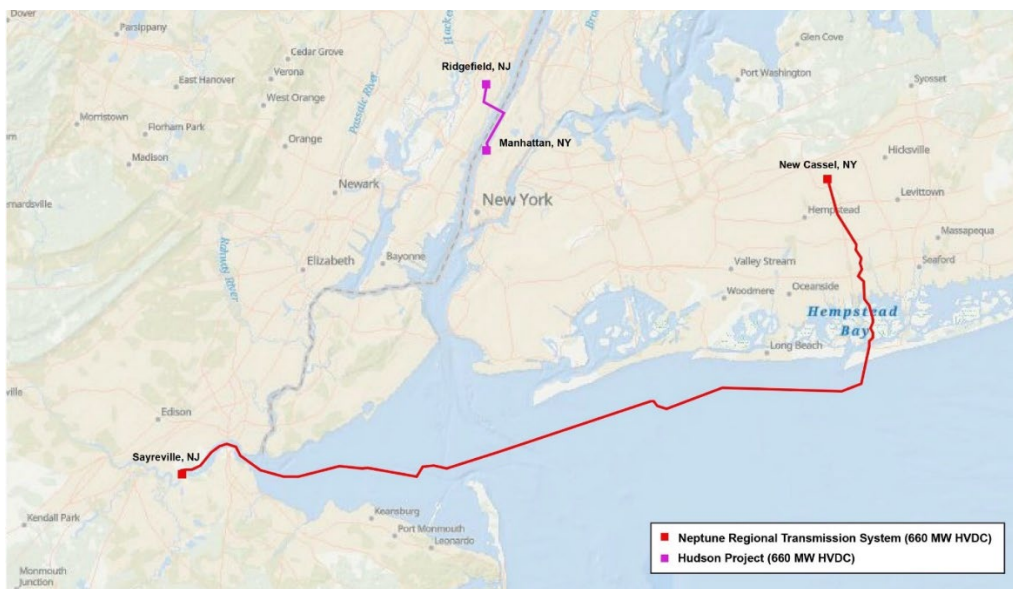
Figure 1-1 Neptune Project and Hudson Project routes
